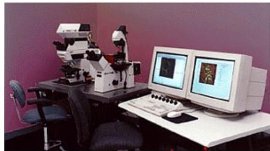
There are two separate microscopes (upright and inverted) that can accommodate the scanning head, which makes the system flexible for various research needs.
